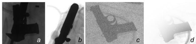
Figure 3: Other problems in recognition of a *gun*: a) occlusion, b) self-occlusion, c) noise, d) wrong acquisition.
