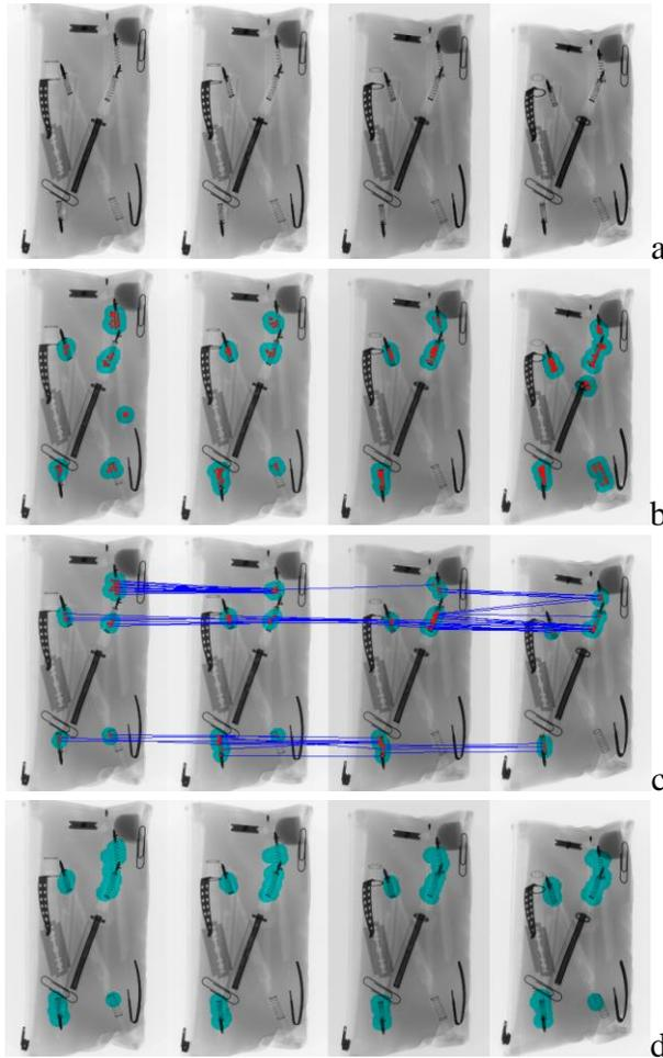
Figure 9: Multiple view detection of springs in a pencil case: a) original test sequence, b) detected monocular keypoints, c) matched keypoints, and d) detection.
