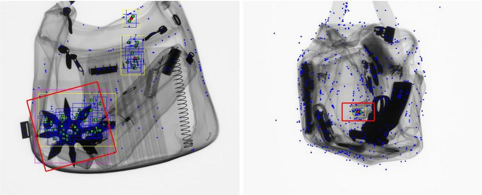
Figure 8: Detection of a shuriken (left) and a razor blade (right) using our approach based on ISM in a single view (see red parallelogram).
