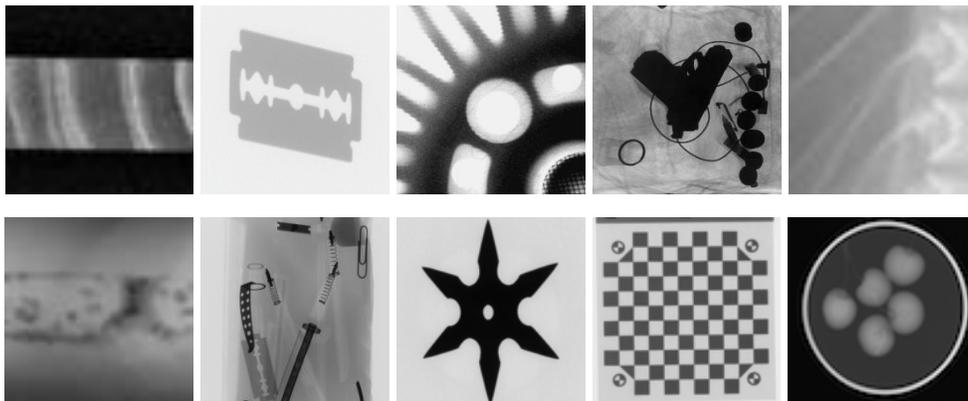
Figure 5: Some X-ray images of our public database GDXray: wood, razor blade, aluminum wheel, bag with a gun, fishbones, weld, pen case, *shuriken*, calibration pattern and apples.
