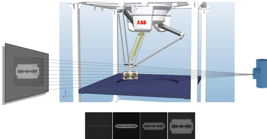
Figure 4: Schematic illustration of our X-ray system: the manipulator can locate the test object in different positions in order to analyze different projections.
