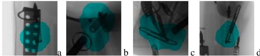
Figure 10: Recognition using our approach in cases with some degree of overlap: a) one spring, b) two springs, c) one clip, d) one clip. Each figure shows a part of one image of the whole sequence.
